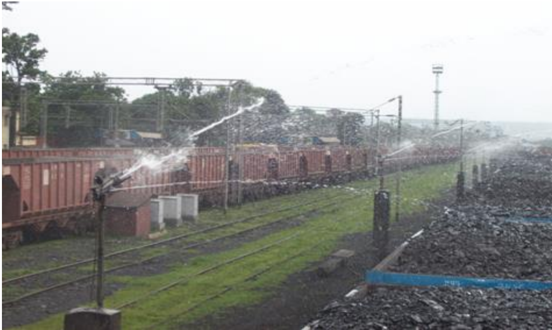
Figure 7.5: Utilization of mine water for water sprinkling in Piparwar OCP, CCL
