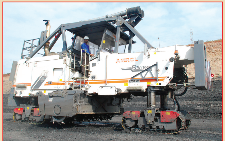
Surface Miner - For Selective Mining
