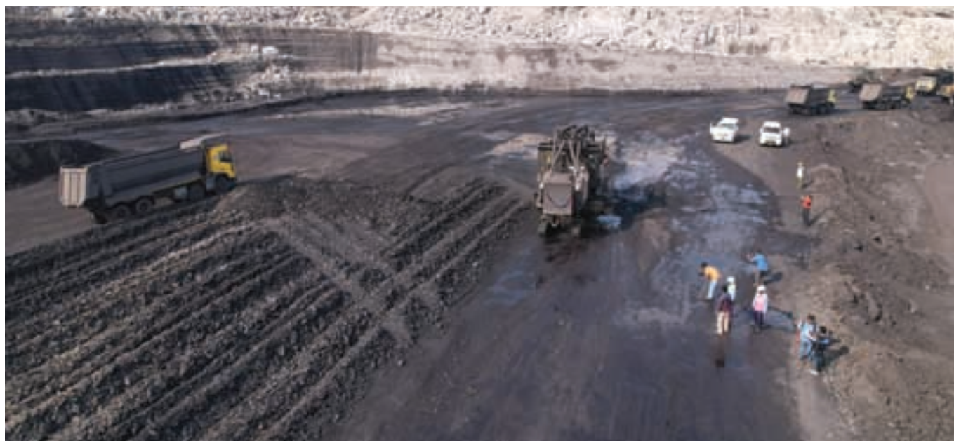
Selective Coal Mining using Surface Miner Technology
