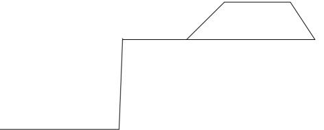
Top width-2.0M , Bottom width-2.0M, Depth-2.0M, Gap between trench and mound-1.0M  $\,$
