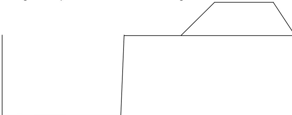
Top width-2.0M , Bottom width-2.0M, Depth-2.0M, Gap between trench and mound-1.0M
