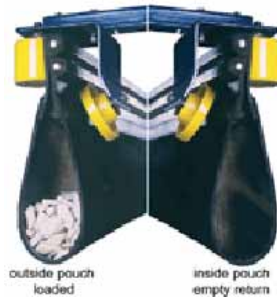
Fig. 14: Cross section of Sandvik's Continuous Haulage system CHS500
