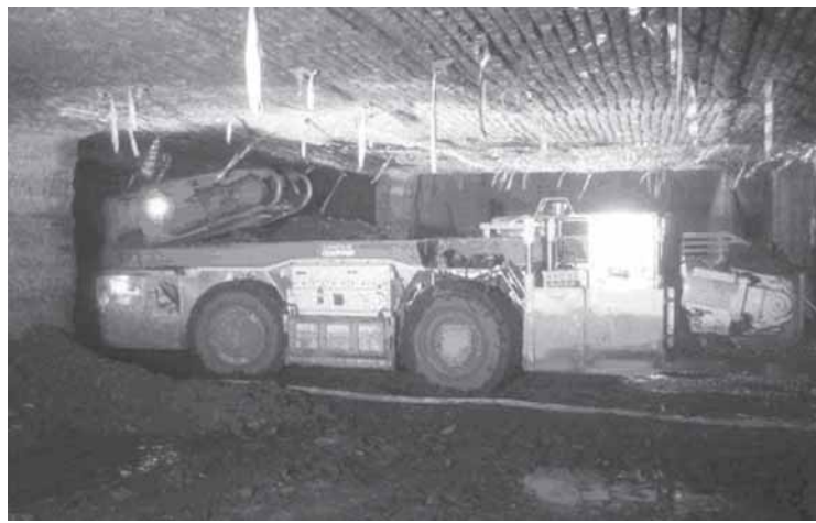
Fig. 12: Shuttle Car TC790 in operation with Bolter Miner
