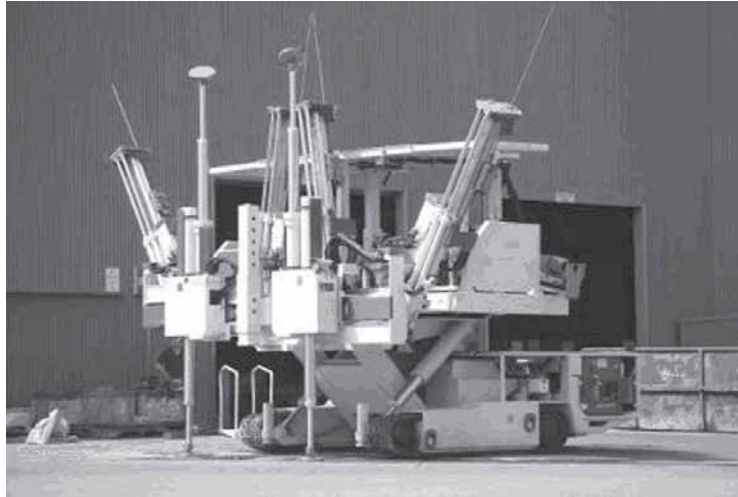
Fig. 9: Mobile bolter DM300 with four roof and two rib bolters
