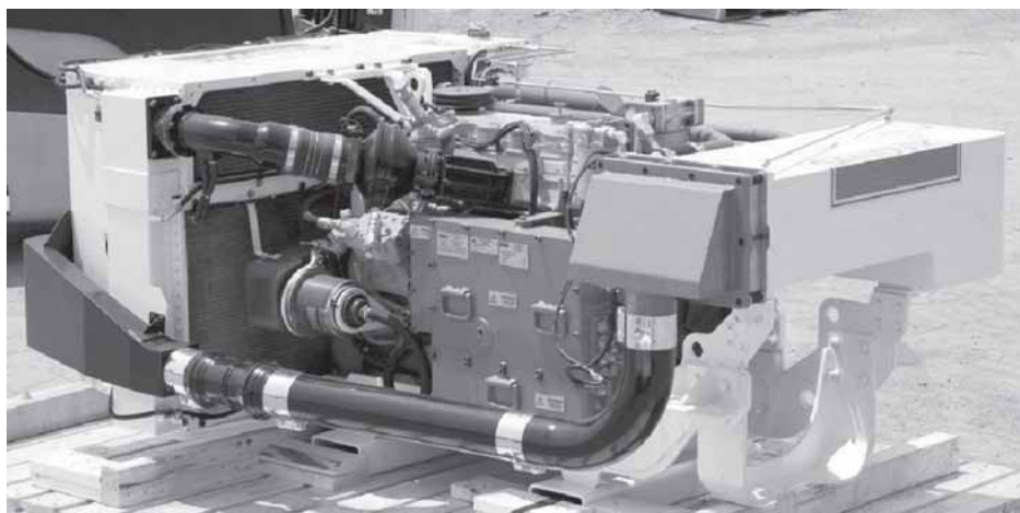
Fig. 4: ATEX approved Diesel engine
