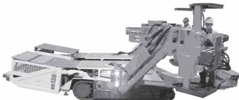
Fig. 8: Mobile bolter DM130 with two bolter operators
