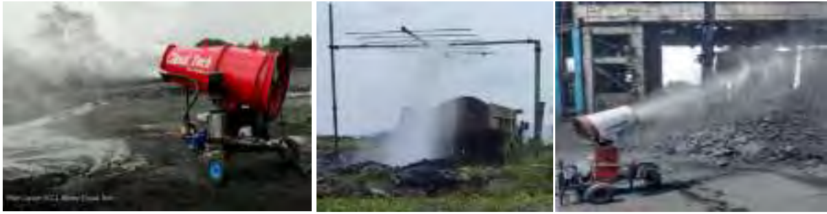
Figure 5.11: Fog cannon deployed at CHP at GK OC, fixed sprinkling at permanent haul roads and mist cannon at CHP at RG OC, SCCL
