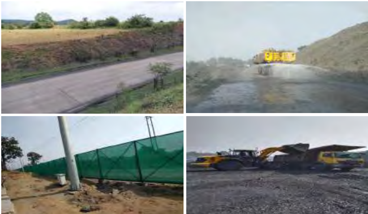
Clockwise from top: (i) Black topping & concreting done on transportation route; (ii) Mobile water sprinklers in operation over haul road; (iii) Installation of green curtains along railway siding; (iv) Use of higher capacity tippers (20-25 tonnes) to reduce trips
