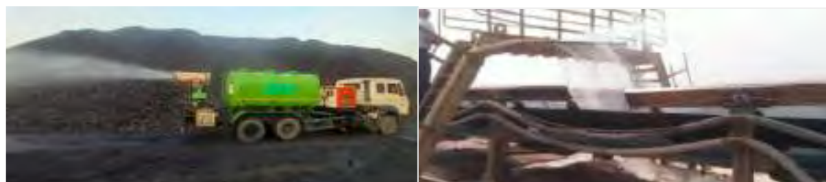
Figure 5.10: Fog cannon along haul roads and water spraying at conveyor belt in Talabira II & III OC, NLCIL
