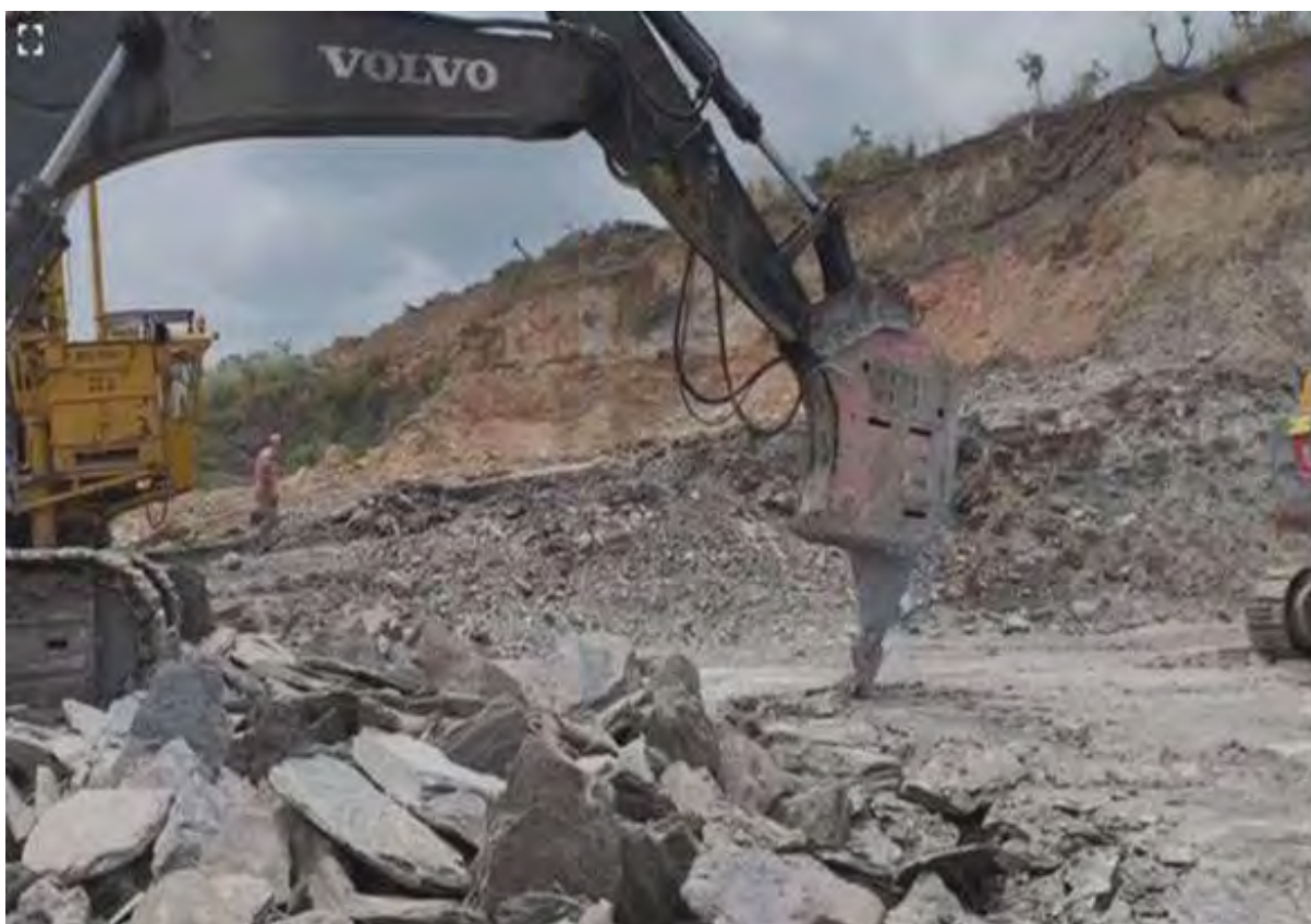
Figure 5.7: Blast-free OB removal at Kaniha OC & Hingula OC of MCL – new initiatives in CIL
