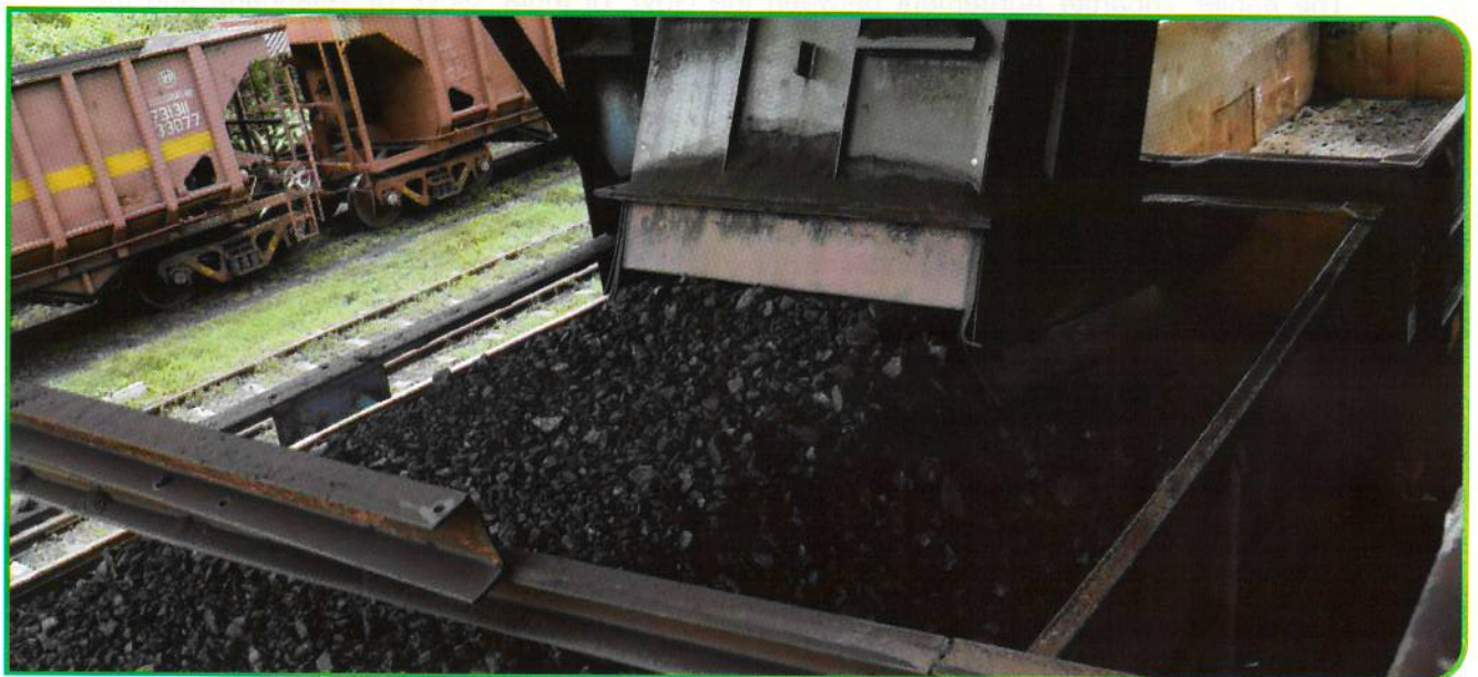
Coal loading into a wagon in Engine on Loading Process at KCHP - Manuguru
