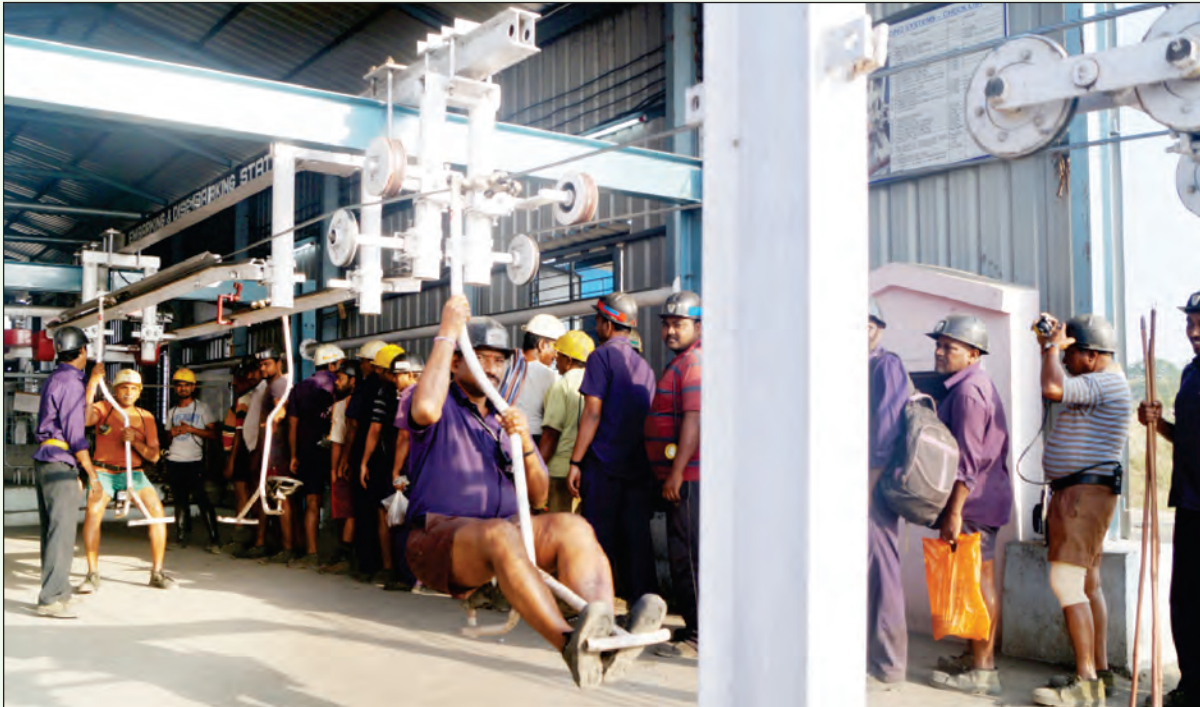
Newly provided Surface Manriding System at Adriyala Longwall project
